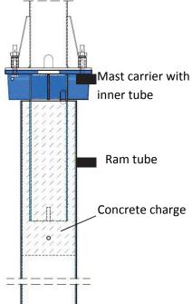
Select the distance between signal mast and track centerline in accordance with the specifications. If the ram tube was rammed in with an offset on account of existing lines, the mast carrier will have to be shifted accordingly within the ram tube.
